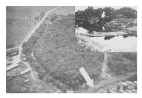
Figure 4-6. Cutoff meander, Souris River (USAED, St. Paul). Cutoff bendways can be maintained for wildlife and recreational benefits. (Inset highlights grade control structure with crest elevation sufficiently high to force normal flows through the bend)
