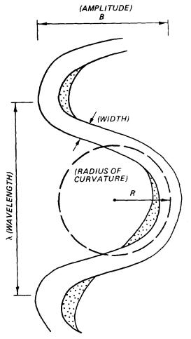
Figure 4-5. Meander geometry
